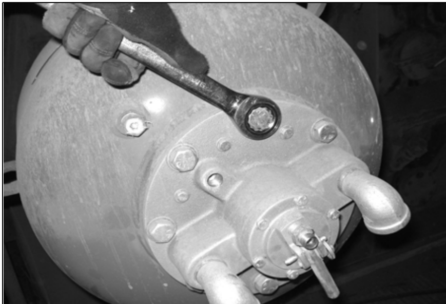
Fig. 15: Removing the screws of the valve
