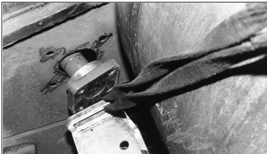
Fig. 6: Alignment of the cleaner shaft (1)
