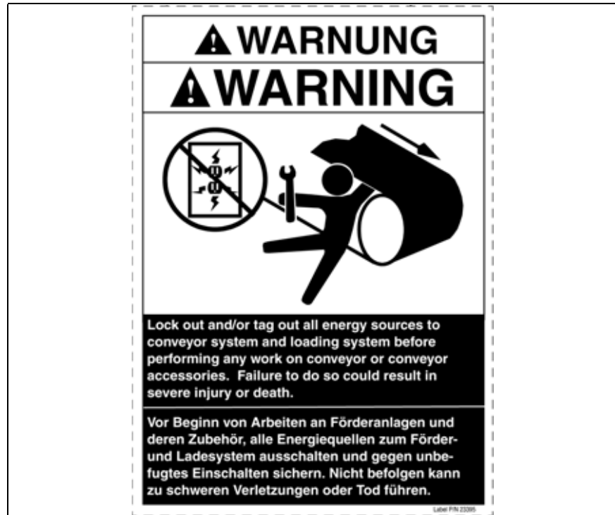
Fig. 27: Warning label for conveyor products, part no.: 23395
