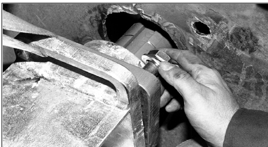
Fig. 7: Alignment of the cleaner shaft (2)
