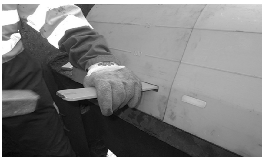
Fig. 23: Driving out the plastic pins
