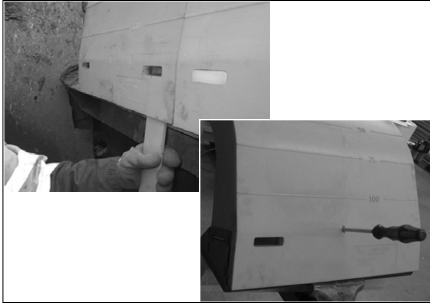
Fig. 24: Drive out the cleaner blade
