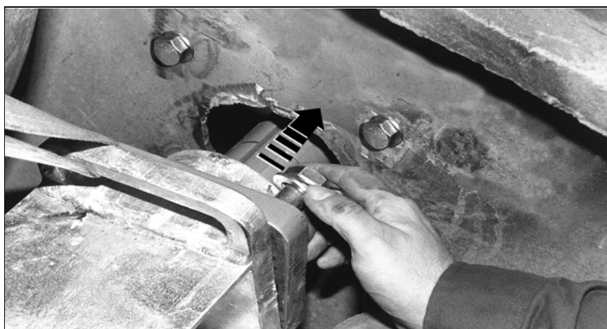
Fig. 20: De-installation of the shaft stub end
