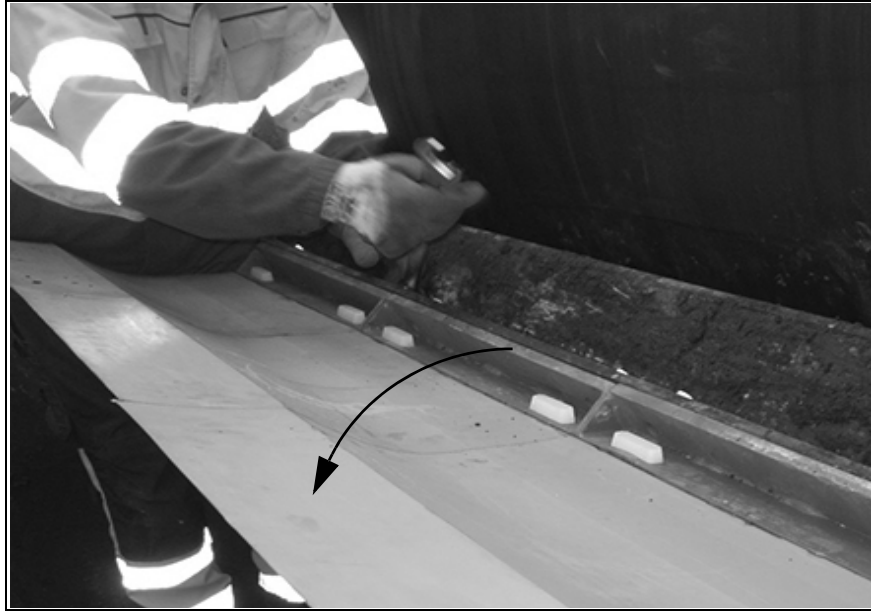
Fig. 13: Final assembly of the blade grip with the cleaner blades
