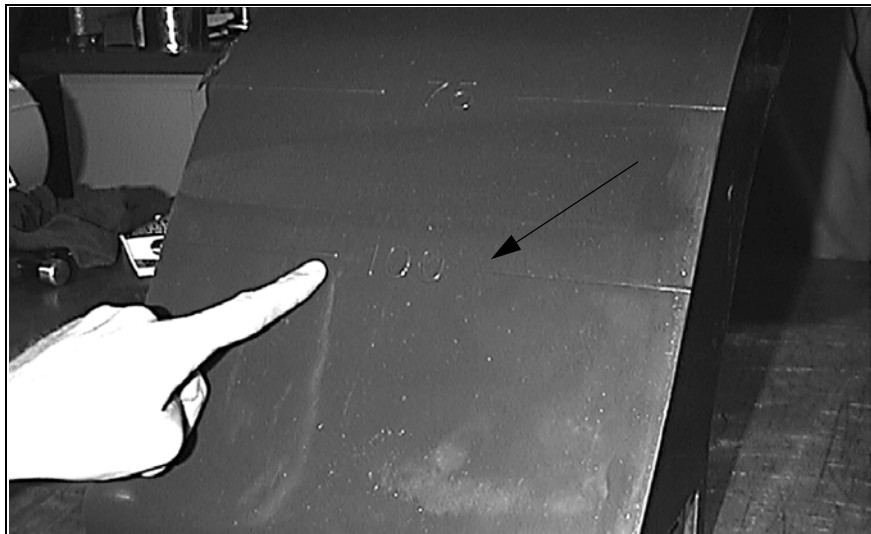
Fig. 19: Illustration of the 100 % wear mark
