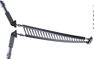
The **CleanScrape® Cleaner** is mounted diagonally on the discharge pulley and forms a three-dimensional curve. The cleaner has a matrix of carbide scrapers incorporated into the main rubber body during the vulcanization process. Despite a relatively low contact pressure between the belt and cleaner 85 to 95% of the adhering material is removed.
