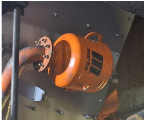
Martin® Hurricane Air Cannon improve the flow of bulk materials
