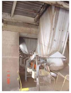
At the Sokolovská Uhelná Mine, Martin® Impact Cradles have more than three years of service in absorbing the impact of large lumps of brown coal dropping more than 20 feet (7 meters).
