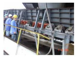
Martin® ImpactCradles were installed at the Sokolovská Uhelná Coal Mine to cushion the impact of falling lumps and to reduce damage to conveyor components.
