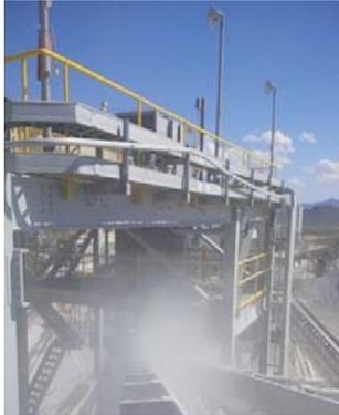
*A mine in north central Mexico was experiencing dangerous spillage at the loading zone of its tower mounted conveyor.*
