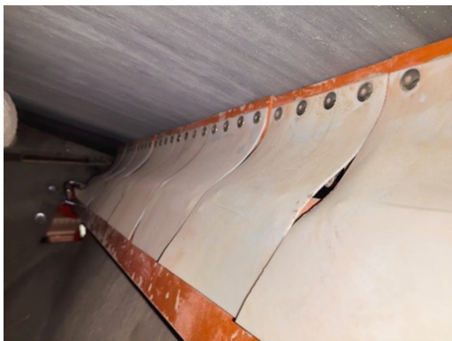
The blade shield ensures smooth discharge of the cleaned material without accumulation.
