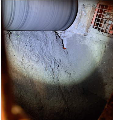
Persistent carryback on most of the conveyors led to excessive cleaning demands & operational challenges.
