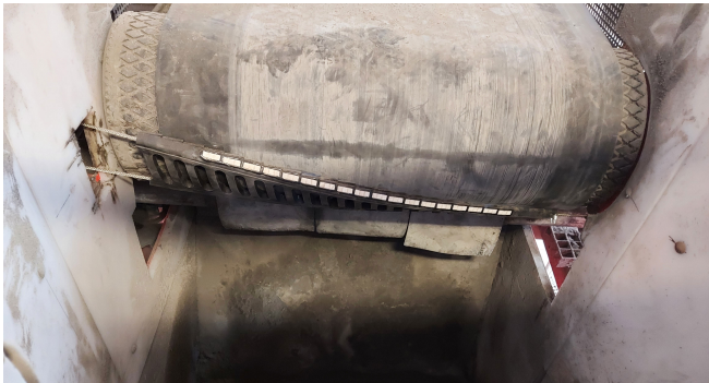
CleanScape® Primary Cleaner installed diagonally for high-efficiency belt cleaning with minimal belt wear
