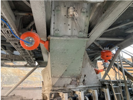
Conveyor systems at gold mines demand for flow-aid systems to maintain material flow & plants performance.
