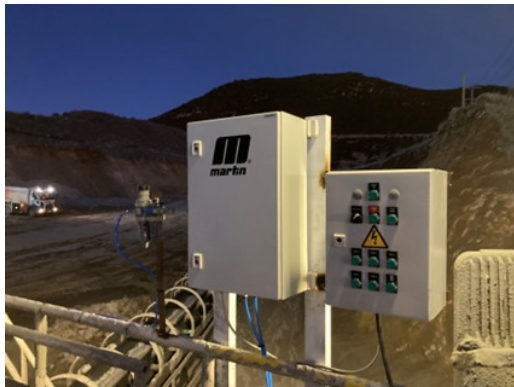
Martin® Hurricane Air Cannon Controller allows adjusting the firing schedule as per de-clogging needs.
