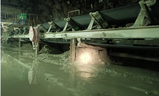
Underground belt conveyors faced carryback issues, resulting in unplanned downtime & potential safety risks.
