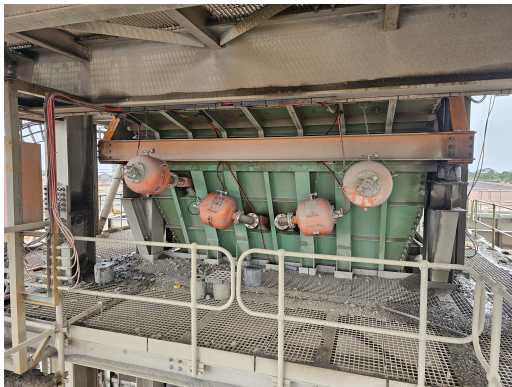
15 numbers of 70-Ltr Martin® Hurricane Air Cannons were strategically installed across critical chutes
