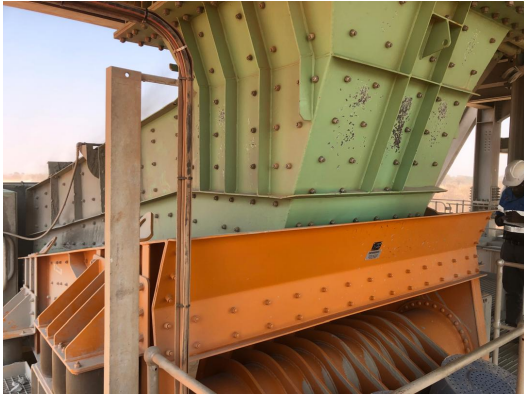
Material build-up in hoppers and chutes often led to manual hammering, causing damage & safety concerns
