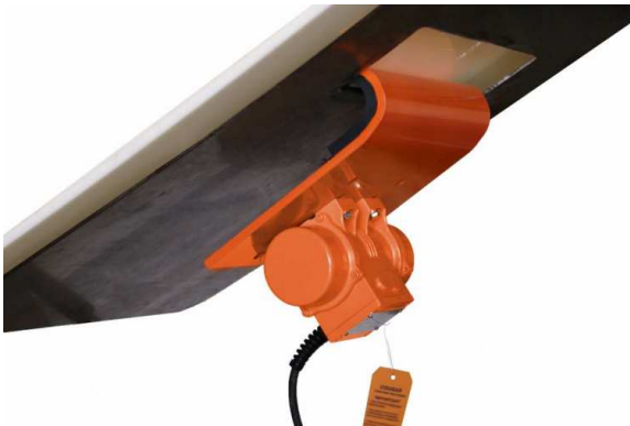
Martin® Vibrating Dribble Chute prevents material from clogging chutes and burying belt cleaners.
