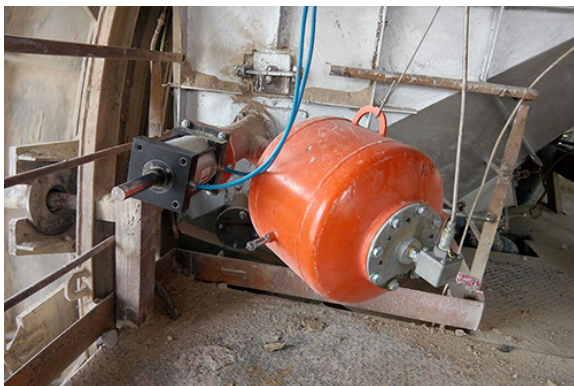
The retractable nozzle is for the most punishing areas where heat and debris quickly reduce equipment life.
