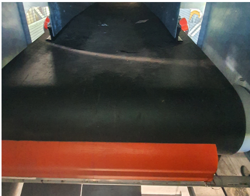
Martin® QC1™ Primary Cleaner HD enhanced belt cleaning efficiency while reducing maintenance costs.
