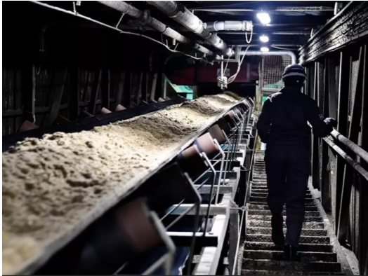
Bagasse material handling poses dust explosions risks, requiring ATEX-compliant equipment to ensure safety.
