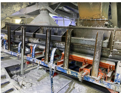
A brush cleaner controls any fines trapped in cracks and divots in the belt from carryback, reducing dust.
