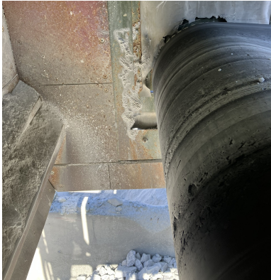
Persistent carryback accumulated along the return belt
