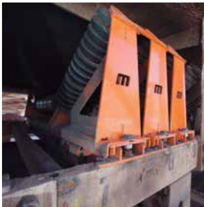
Figure 2. The new EVO high-speed roller cradle employs multiple heavy-duty impact rollers spaced close together in a track-mounted configuration.
