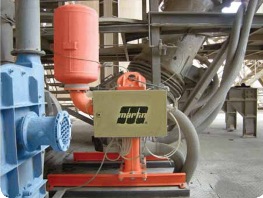
Figure 2: Martin Engineering has introduced two multiple-port air cannon systems that use a single reservoir and control unit to replace up to eight traditional tank-and-valve air cannons
