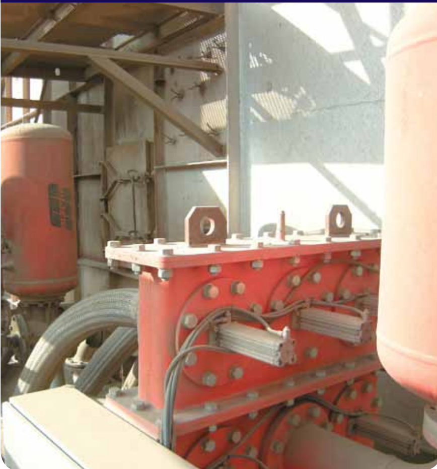
Figure 3: the Martin® Multi-Port Air Cannon System delivers its air blast to as many as eight ports without conventional valves, using air cylinders designed to operate for millions of cycles without maintenance
