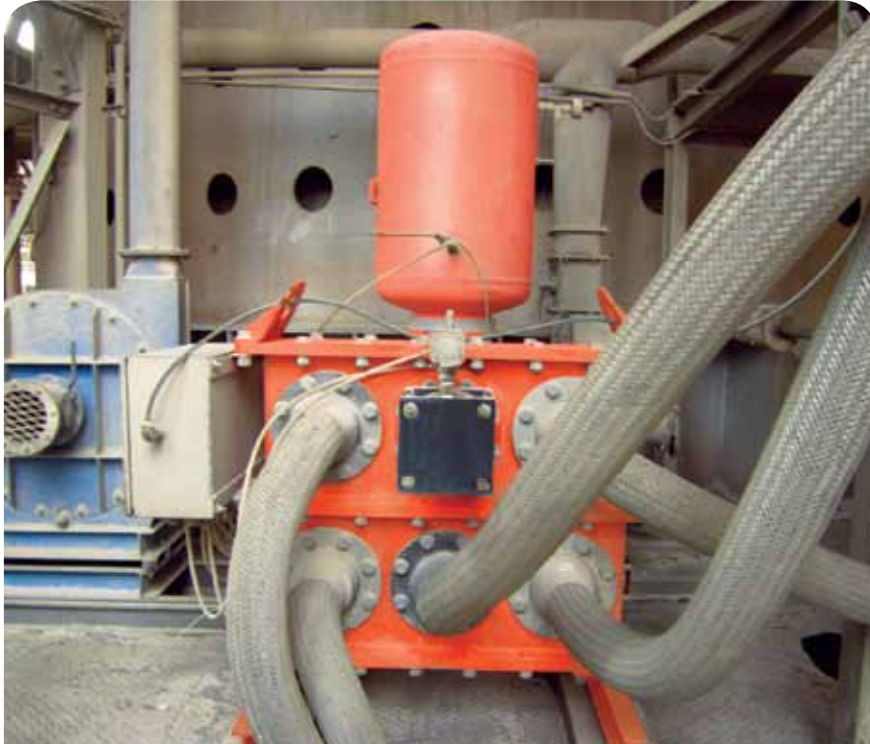
Figure 3: with a single air tank discharging through stainless steel hoses and/or rigid pipes, multiple-port systems separate the air cannon valves from the discharge points, protecting components from heat, contaminants, high pressure washing or cordox
