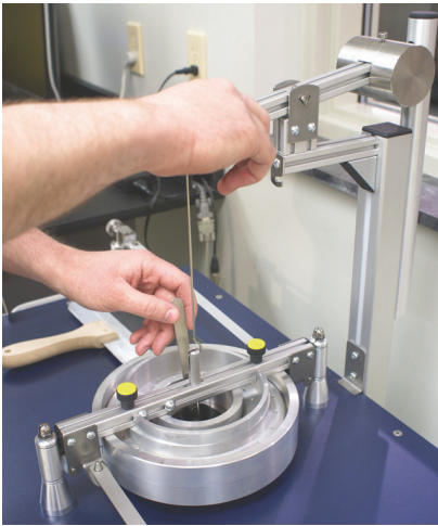
CFI ring shear tester: the ring shear tester is used to measure the flow properties of powders and bulk solids.
