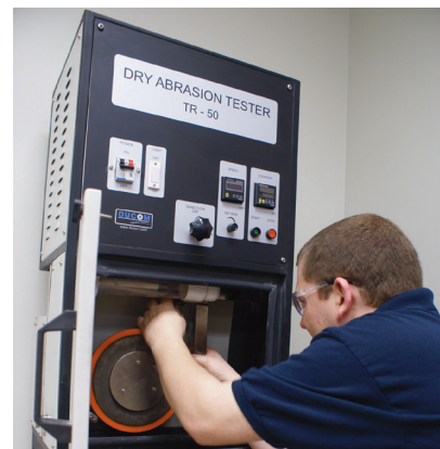
A dry abrasion tester checks three-body abrasive wear, as between a conveyor belt, a metal chute liner and the bulk material.
