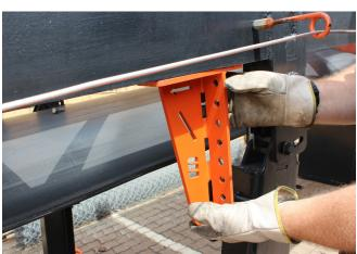
**STEP 4:** Ensure brackets is facing the correct way (arrow to point in the direction of the return belt).
