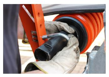
**STEP 8:** Loosly fasten the MRT using the U-bolts equally on both brakcets.
