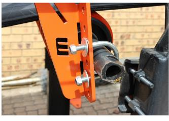
**STEP 10:**Securely fasten all bolts, nuts and U-bolts.
