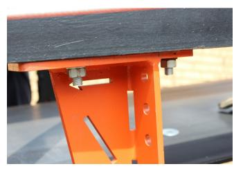
**STEP 6:**Set height of MRT approximately 5mm higher than the removed return idler.
