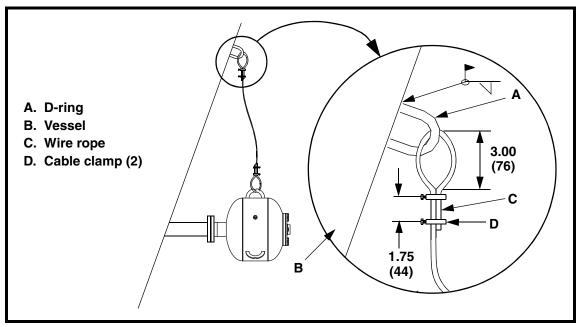
Figure 14. Installing Restraining Cable
