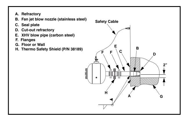
**Figure 9. Installing Mounting Plate (High-Temperature Applications)**
