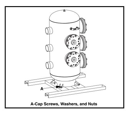
Figure 15. Installing Air Cannon System
