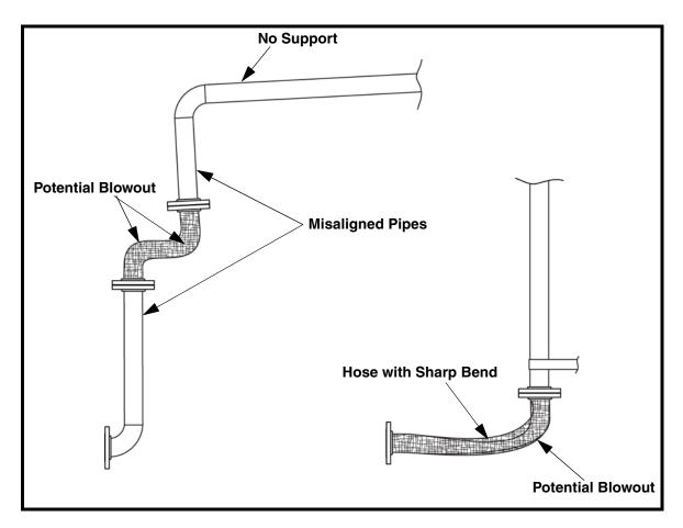
Figure 13. Improper Hose and Pipe Installation
