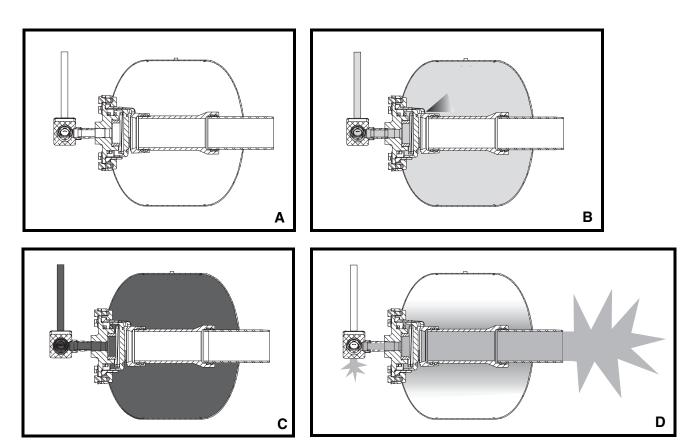
Figure 2. Air Cannon Charging and Discharging
