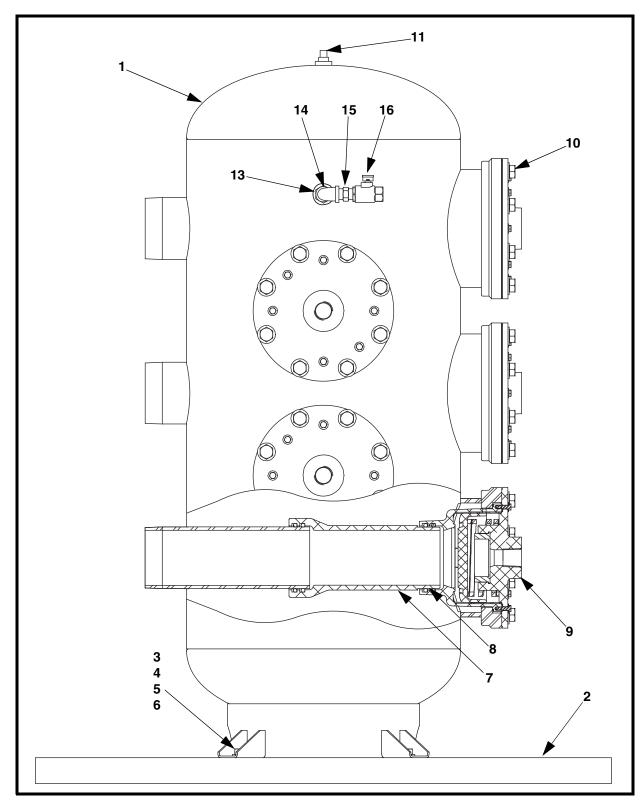
Figure 20. Martin<sup>®</sup> Multi Valve Air Cannon System Parts List, P/N 38625-FD
