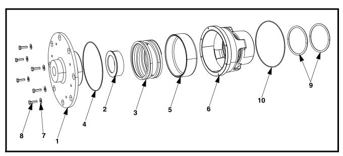
Figure 19. Martin<sup>®</sup> Typhoon Air Cannon Valve Assembly Parts List, P/N 38071-FD
