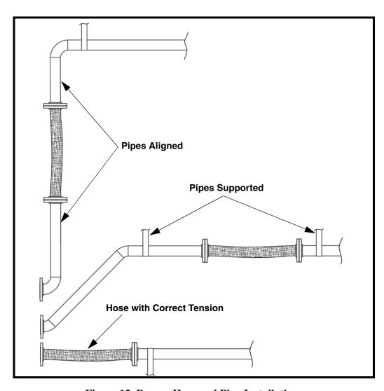
Figure 12. Proper Hose and Pipe Installation
