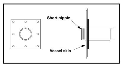
Figure 5. Standard Mounting Plate
