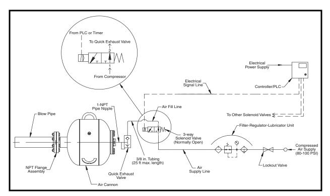
Figure 16. Solenoid Enclosure Piping
