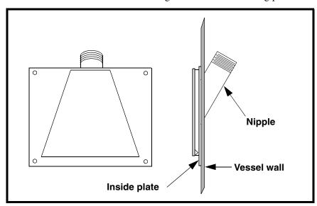
Figure 7. Fan Jet Mounting Plate
