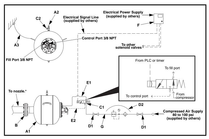
Figure 16. Plumbing Detail for Normally-Opened Solenoid Valve
