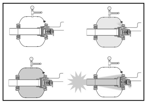
Figure 1. Air Cannon Charging and Discharging
