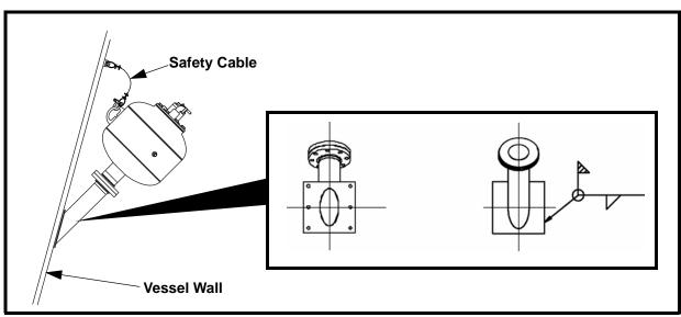
Figure 3. Installing 30-Degree Mounting Plate
