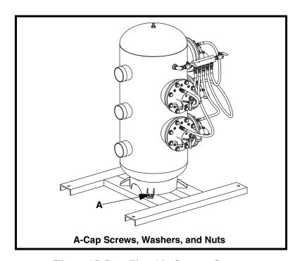
Figure 15. Installing Air Cannon System
