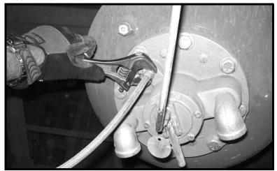
4. Remove the 8 bolts on the valve assembly.
