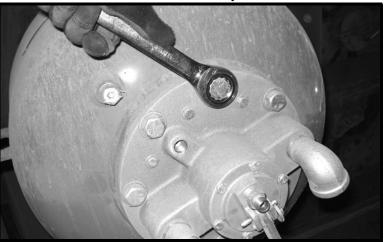
5. Remove valve from tank. A small pry bar can help if O-rings are dry.
