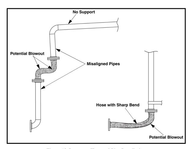
Figure 13. Improper Hose and Pipe Installation
