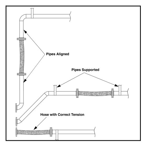
Figure 12. Proper Hose and Pipe Installation
