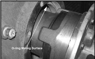
11. Install the 8 cap screws and compression washers.
