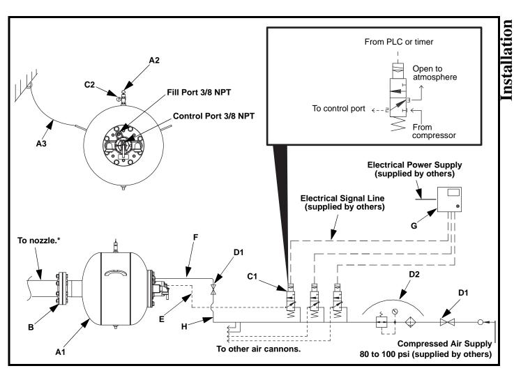
Figure 17. Plumbing Detail for Normally-Closed Solenoid Valve
