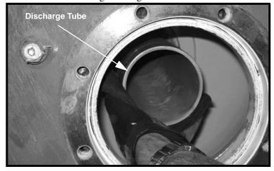
10. Mate the valve assembly back onto discharge tube, making sure not to pinch O-ring.
