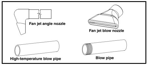
Figure 5. Mounting Nozzles/Pipes for High-Temperature Applications
