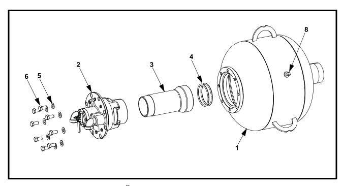
Figure 18. Martin<sup>®</sup> Hurricane Air Cannon Assembly Parts List
