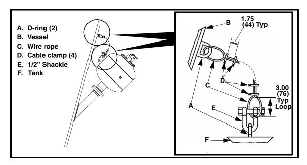
Figure 14. Installing Restraining Cable
