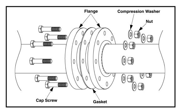
Figure 11. Flange Installation
