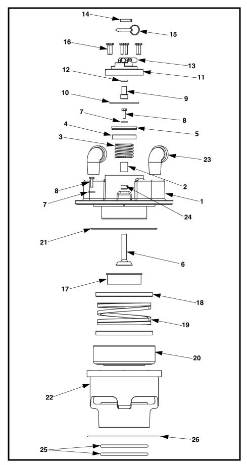
Figure 19. Martin<sup>®</sup> Hurricane Air Cannon Valve Assembly Parts List, P/N 38071
