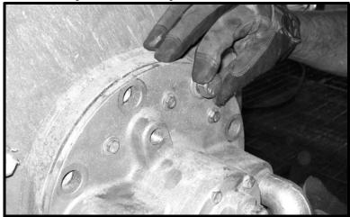
12. After the valve assembly is bolted to tank, re-connect air lines. Ensure there are no leaks or loose connections.
