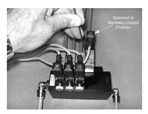
3. Rotate solenoid 180 degrees. Reinstall screws and tighten. Repeat this procedure for each solenoid to place all solenoids in the normally-closed position.
