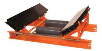
The EVO® Slider Cradle utilizes low friction UMHW bars to support the belt at the outside of the load-carrying area. This stabilizes the belt line, eliminating the sag and bounce that spill material, and reducing the risk of catching lumps that can abrade the belt surface.
