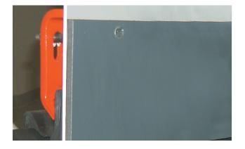
Installed inside conveyor transfer point skirtboards, <u>Martin</u><sup>®</sup> <u>Wear Liner</u> creates a dam to shield the sealing system from the weight of the material load, prolonging the life of the seal.
