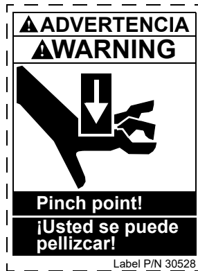
Figure 8. Pinch Point Warning Label, P/N 30528
