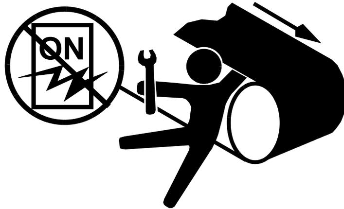
**Lock out and/or tag out all energy sources to conveyor system and loading system before performing any work on conveyor or conveyor accessories. Failure to do so could result in severe injury or death.**
