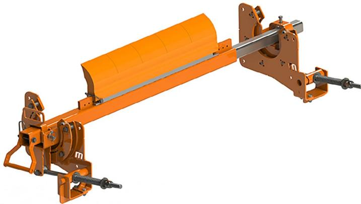
The [Martin® QC1™ Cleaner HD STS](#) tackles the tough jobs. Designed for rugged conditions, this sturdy cleaner's stainless steel mandrel allows the blade cartridge to be serviced without confined space entry or breaking the safety plane. Changing the blade is a simple one-pin operation, making replacement of a worn blade a safe and simple procedure.
