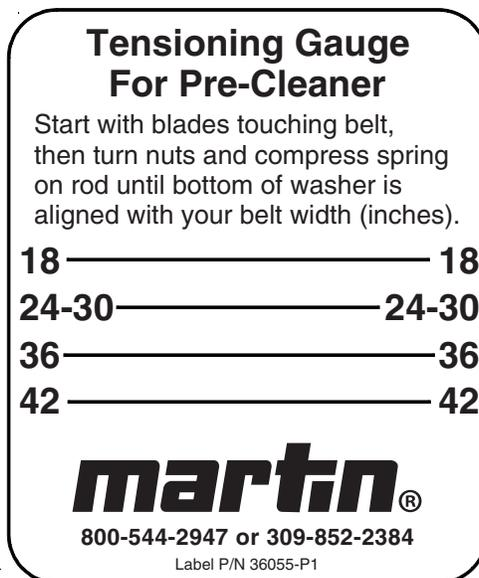
Figure 6. Martin<sup>®</sup> Spring Tensioner XHD Label, P/N 36055-P1
