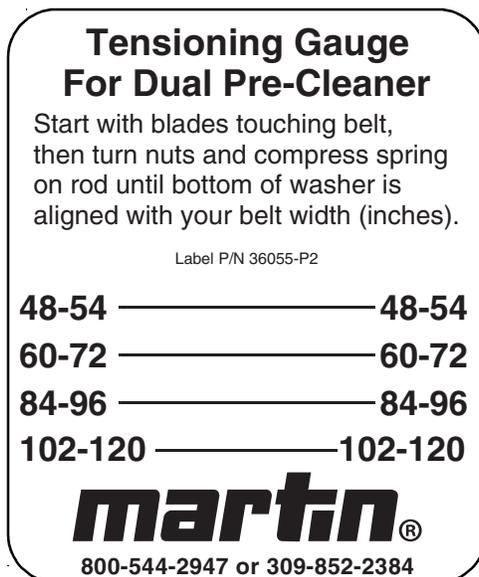
Figure 7. Martin<sup>®</sup> Spring Tensioner XHD Label, P/N 36055-P2
