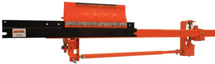
The [Martin® SQC2S™ Cleaner STS](#) incorporates individually-cushioned tungsten carbide blades for effective cleaning without risk to belt, splice, or blade. Installed in the secondary cleaner position, the Martin® SQC2S™ Cleaner's blade buffers cushion impact and maintains cleaning pressure. This cleaner's extended cartridge allows the blade cartridge to be serviced without confined space entry or breaking the safety plane.
