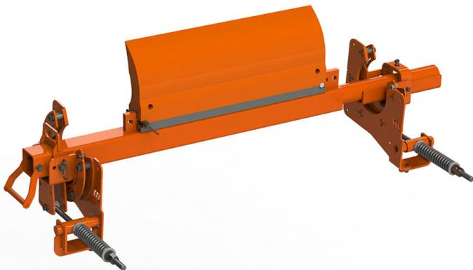
The [Martin® QC1™ Cleaner XHD STS](#) tackles the tough jobs. Designed for rugged conditions, this sturdy cleaner's stainless steel mandrel allows the blade cartridge to be serviced without confined space entry or breaking the safety plane. Changing the blade is a simple one-pin operation, making replacement of a worn blade a safe and simple procedure.
