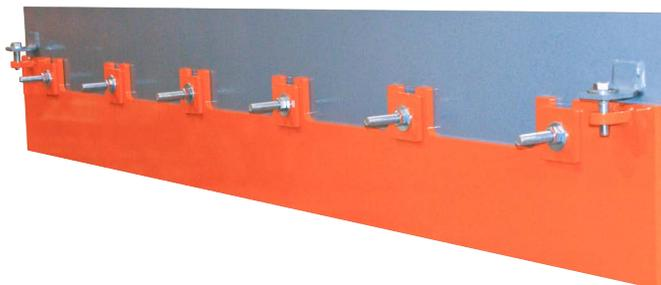
Installed outside conveyor transfer point skirtboards, [EVO® External Wear Liner Retrofit Kit](#) is an economical upgrade that improves skirtboard sealing and prevents spillage. Wearliner can typically be installed without requiring work inside chute or interfering with existing chute supports.
