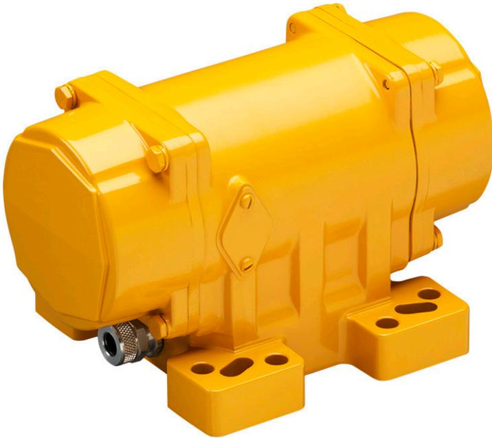
**Cougar® DC Truck Vibrators** solve problems in the unloading of material from mobile equipment. Powered by either 12 or 24-volt DC, the Cougar® Model MDC12-400/700 provides effective vibration to improve material movement. These heavy-duty vibrators are suitable for applications such as concrete pumps, fertilizer, gravel, sand and salt-spreaders, dump trucks and other mobile equipment where sticky or compacted material causes hang-ups and slow unloading.
