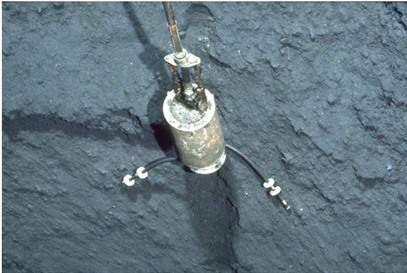
*The Martin® Heavy Duty Whip is used to safely and quickly remove hardened, non-flowing material from silo walls and feeders.*
