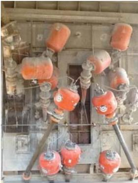
*The Martin® Air Cannons were designed to fit in smaller places, providing more power from less air.*
