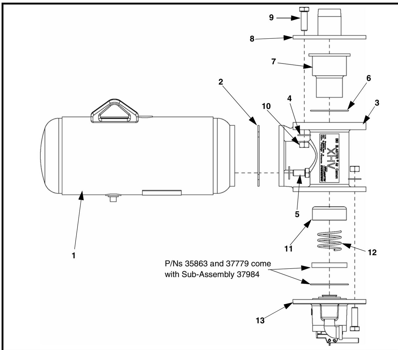
Figure 14. Martin® Tornado Air Cannon 2” Assembly, P/N 37864-XXXX\*
