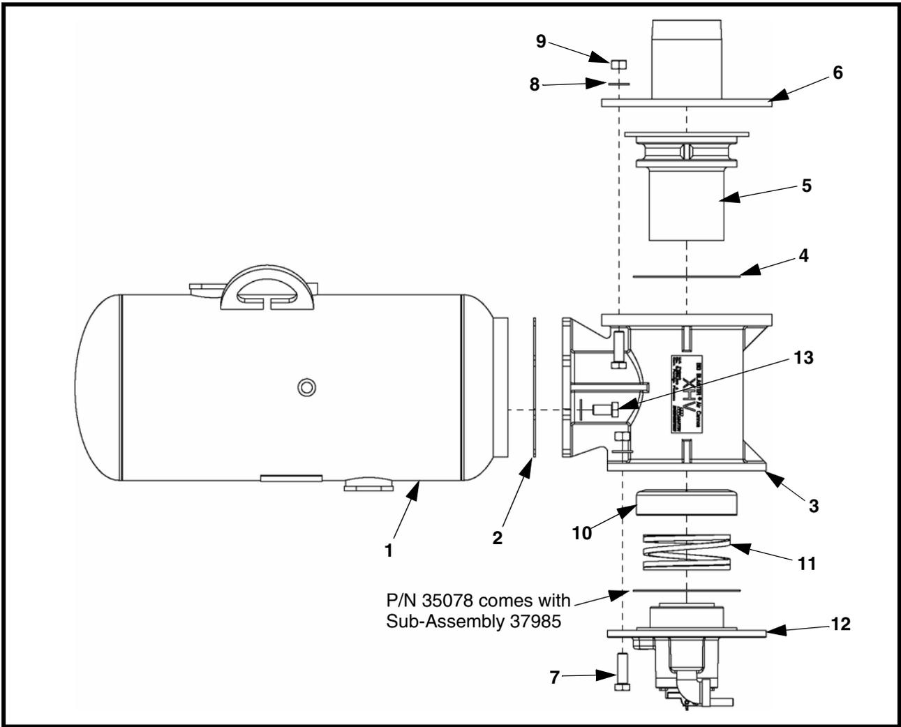
Figure 15. Martin® Tornado Air Cannon 4” Assembly, P/N 37798-XXXX\*
