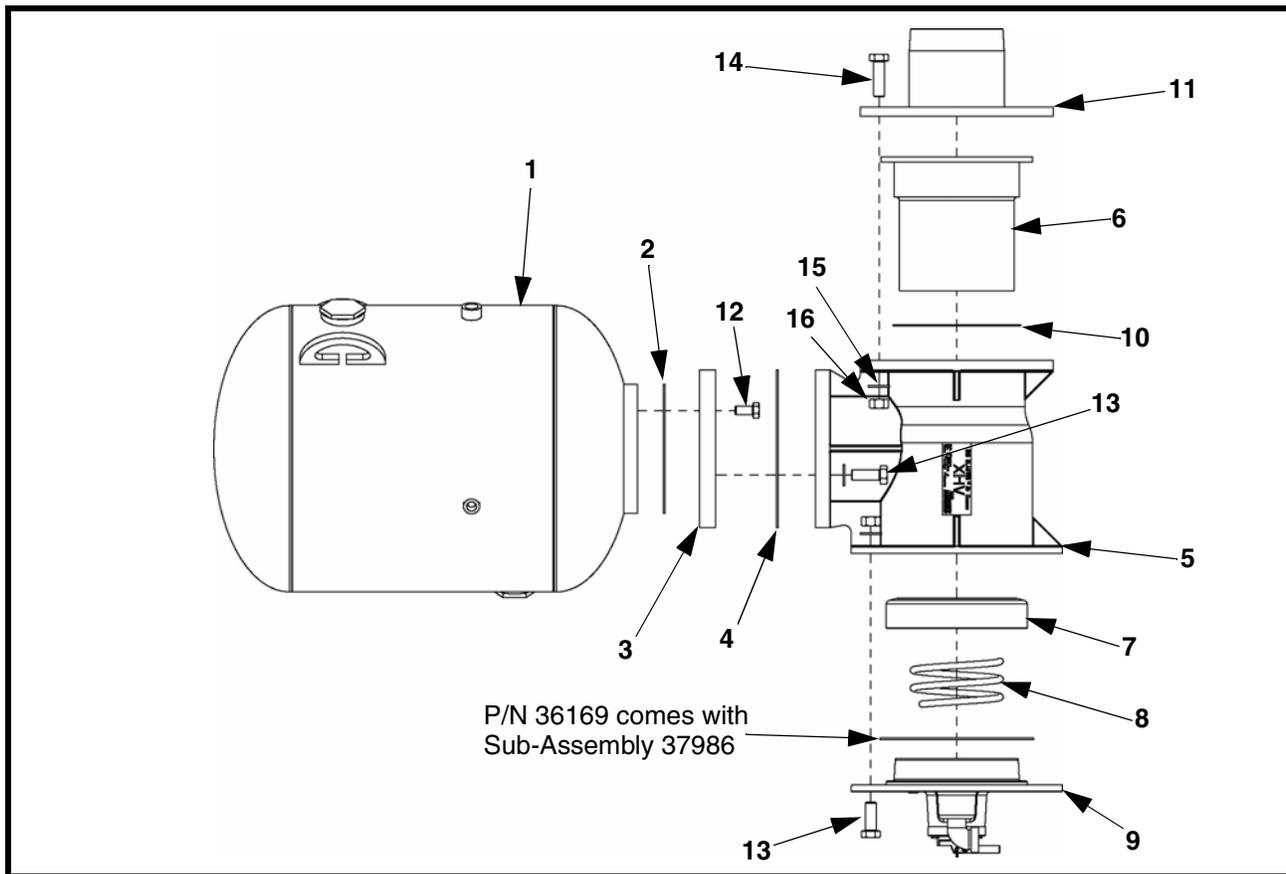
**Figure 16. Martin® Tornado Air Cannon 6” Assembly, P/N 37853-XXXX\***
