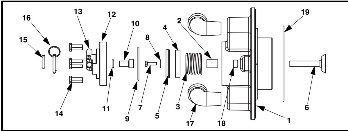
Figure 19. Martin® Tornado Air Cannon Exhaust Valve, P/N 37986
