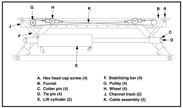
Figure 9. Replacing Cable Assembly
