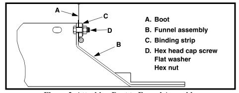
Figure 2. Attaching Boot to Funnel Assembly
