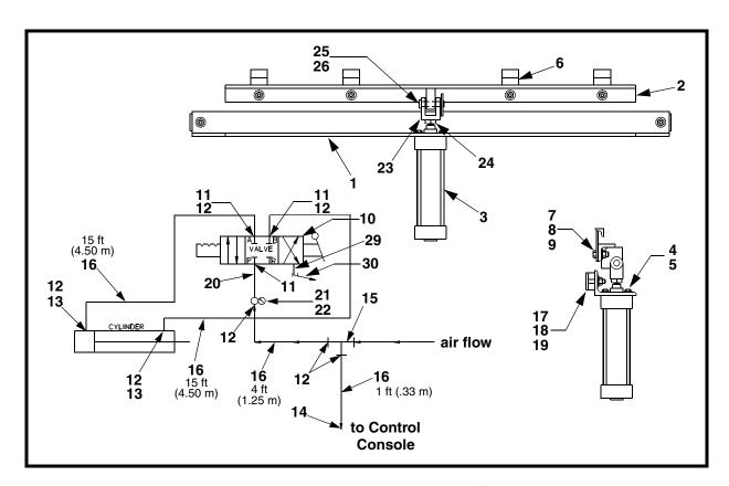
Figure 13. Pneumatic Aligner Assembly, P/N 34140-XX
