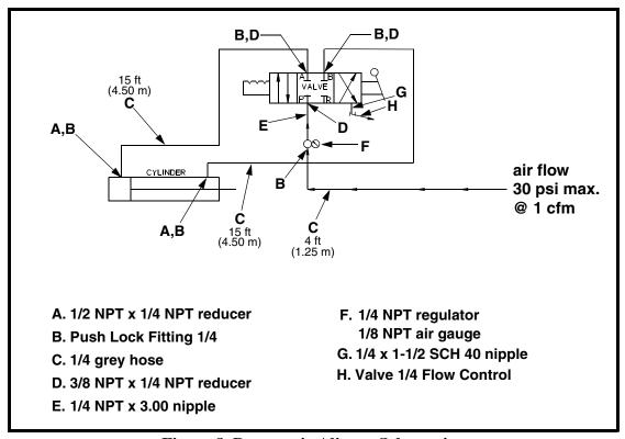
**Figure 8. Pneumatic Aligner Schematic**
