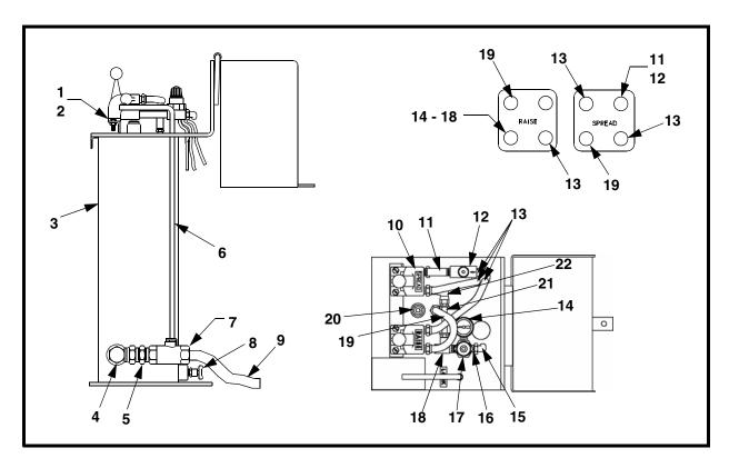
Figure 11. Boot-Lift® DBL-18 Control Console, P/N 38340X-DBL\*\*
