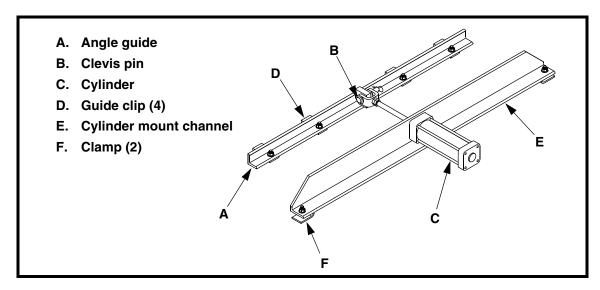
Figure 7. Installing Pneumatic Aligner
