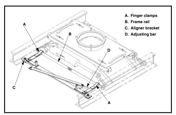
Figure 6. Installing Manual Aligner
