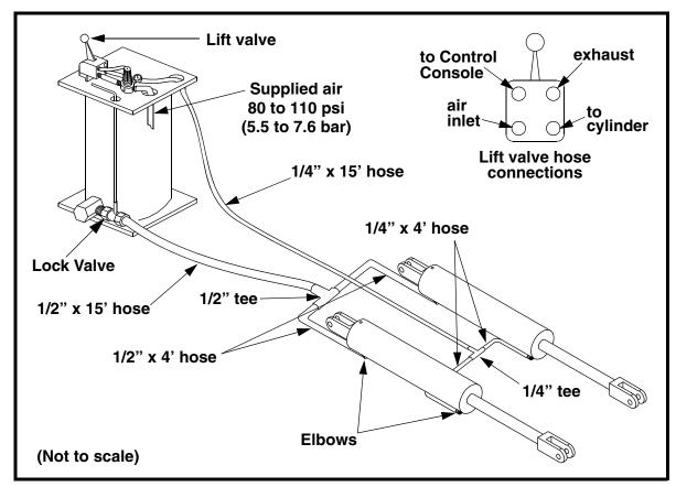
Figure 3. Hose Connections for Models SBL-18, SBL-24, SBL-30, and SBLR-18
