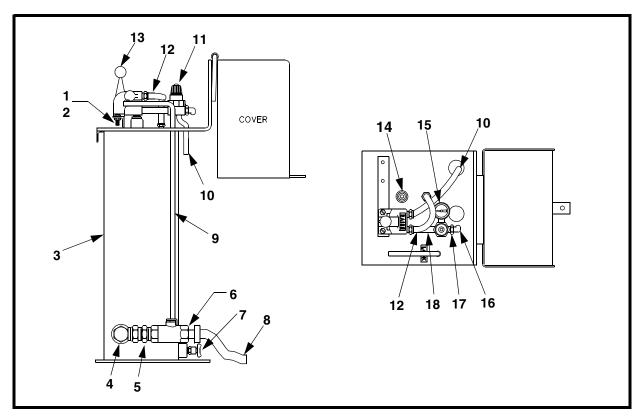
Figure 12. Boot-Lift® Control Console Assembly, P/N 38340X-SBL
