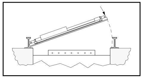
Figure 5. Positioning Railcar Connector on Rails
