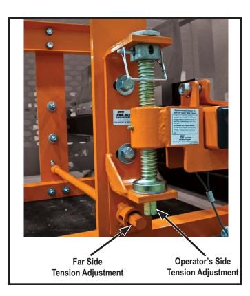
The <u>Martin<sup>®</sup> SQC2S<sup>™</sup> Cleaner STS</u> incorporates individually-cushioned tungsten carbide blades for effective cleaning without risk to belt, splice, or blade. Installed in the secondary cleaner position, the Martin<sup>®</sup> SQC2S<sup>™</sup> Cleaner's blade buffers cushion impact and maintains cleaning pressure. This cleaner's extended cartridge allows the blade cartridge to be serviced without confined space entry or breaking the safety plane.
