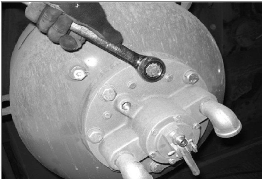
Fig. 15: Removing the screws of the valve
