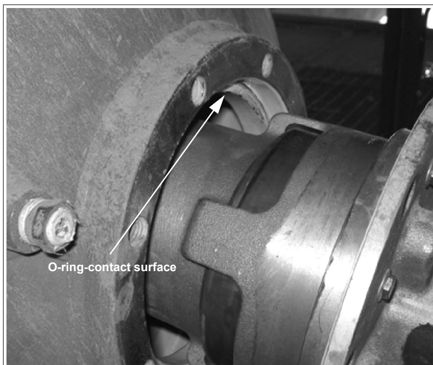
Fig. 20: Insert the valve
