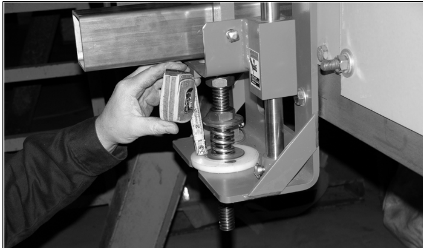
Abb. 12: Spring tensioner - adjusting the spring dimension
