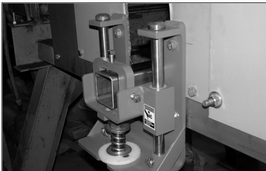
Abb. 4: Arresting the scraper shaft (1)
