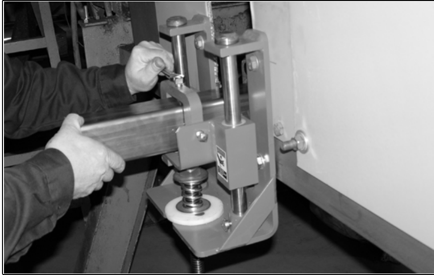
Abb. 5: Arresting the scraper shaft (2)
