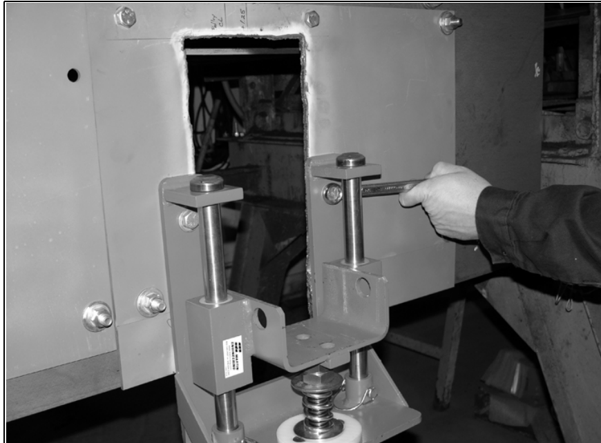
Abb. 2: Installing the installation console with safety bolts
