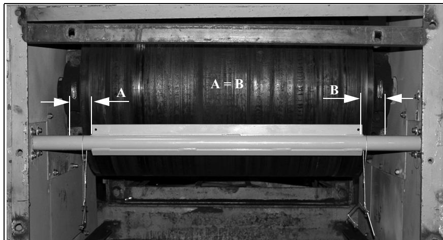
Abb. 8: Centring the conveyor belt scraper shaft (example)
