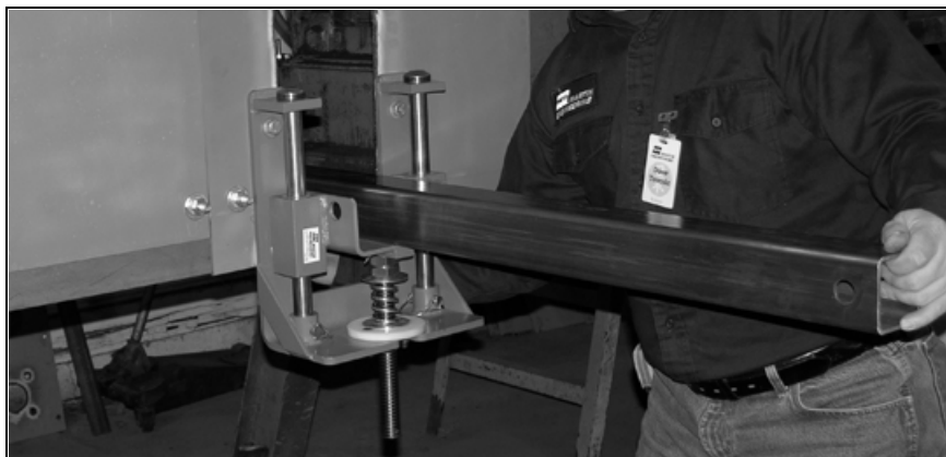
Abb. 3: Sliding in the scraper axis
