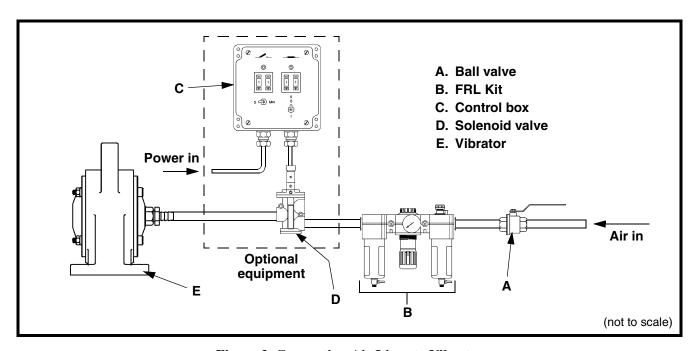
Figure 2. Connecting Air Lines to Vibrator
