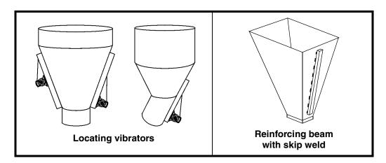
Figure 1. Locating Vibrators and Reinforcing Beams on Hoppers
