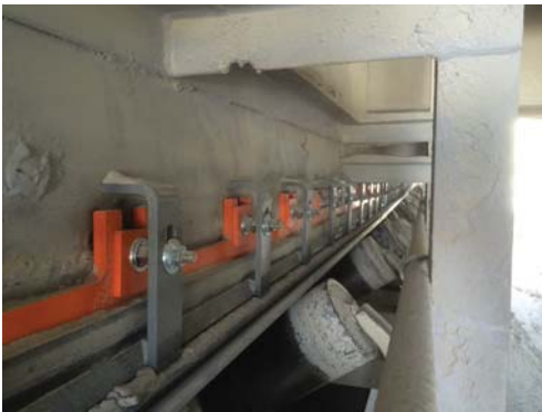
The addition of the external wear liner provided effective sealing.
