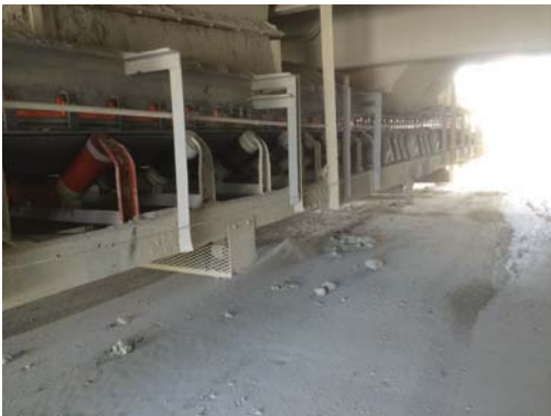
Martin® Trac-Mount™ Idlers utilize sliding frames that will fit in tight spaces allowing for easy installation and service.
