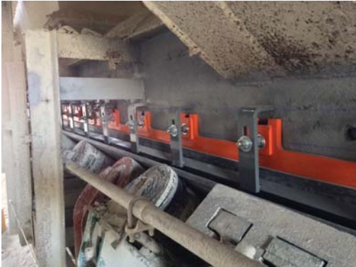
Wear Liner creates a dam to shield the sealing system from the weight of the material load, prolonging the life of the seal.
