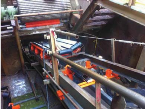
A chemical plant in France was experiencing buildup in their salt storage facility and carryback along the conveyor.
