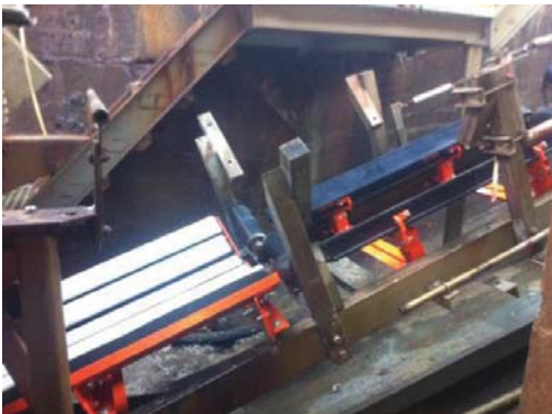
Martin® Slider Cradles were added under the skirtboard of the transfer point to support the edges of the belt.
