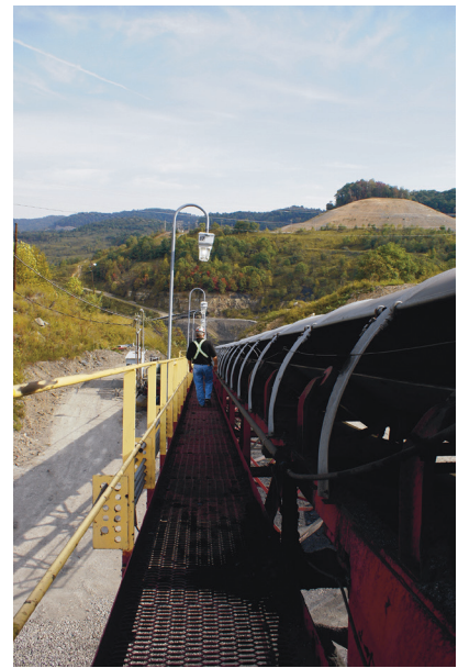
Some suppliers will walk the belt and provide a state-of-the-system report from observing it in operation.
