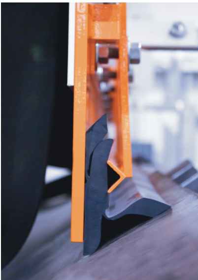
New advances include a skirtboard seal design with a primary seal clamped to the skirtboard and an outrigger strip to capture fines.
