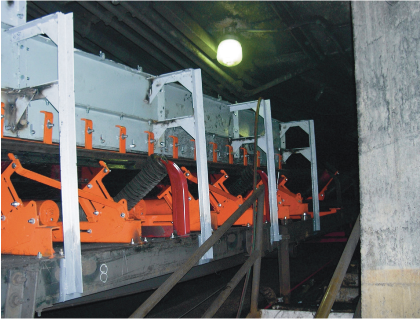
A settling zone controls the air current travelling with the material stream, allowing airborne particles to fall back into the bulk material.
