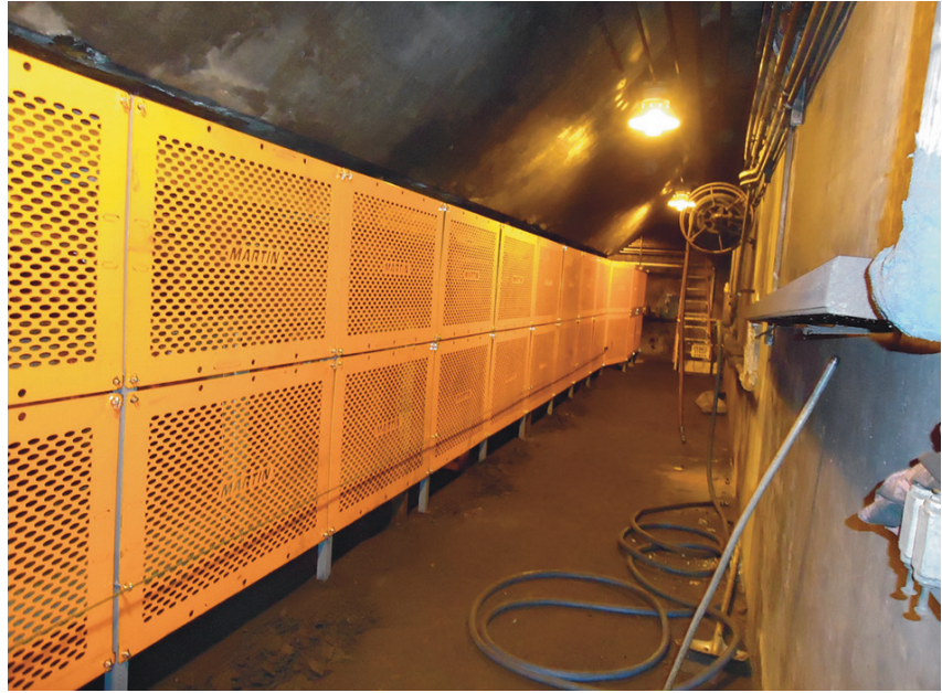
Pinch points should be equipped with well-designed guards to prevent accidental or unwise encroachment by employees or visitors.
