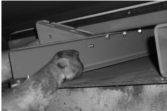
13. Bolt wings in the correct holes but do not tighten.
