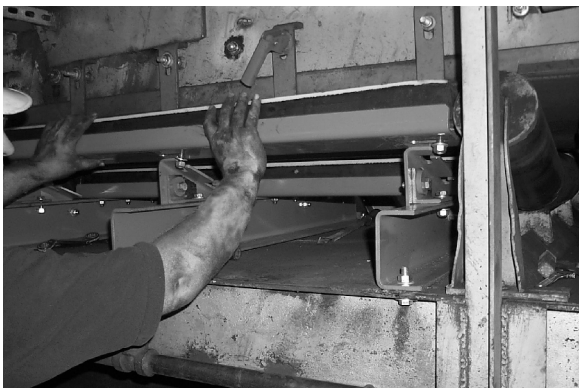
16. Install impact bars on wings.
