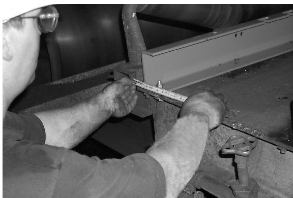
Figure 2. Installing Martin® Impact Cradles
