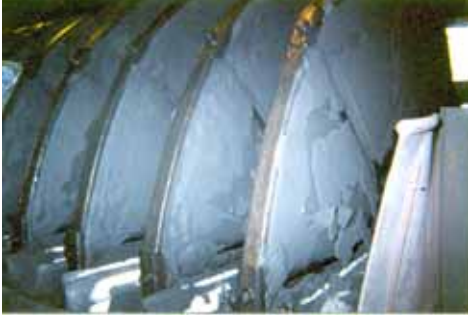
Filter cake is released from the filter sections with the discharge of air from a Martin® Air Cannon.
