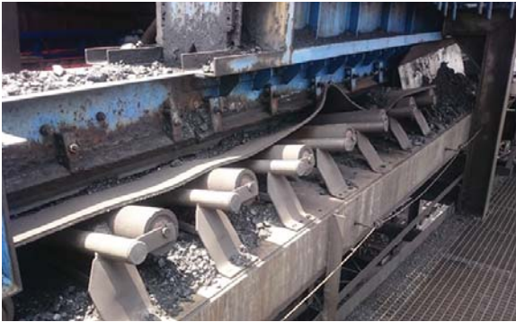
A coal mine in Eastern South Africa was experiencing heavy spillage and system damage due to inadequate loading zone.
