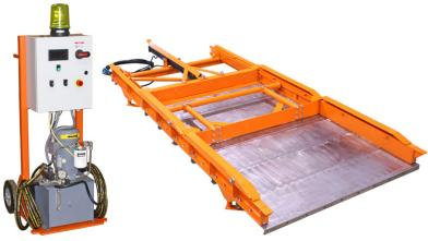
The Martin® Carryback Capture System is designed to return carryback from secondary and tertiary cleaners to the main cargo stream. Carryback from secondary and tertiary cleaners falls into the collecting trough and is pushed back into the material flow by steel cleaning blades.
