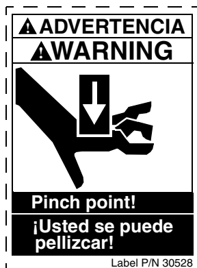
Figure 3. Pinch Point Warning Label, P/N 30528
