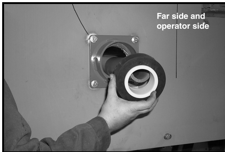
Figure 5. Installing Shock Rings
